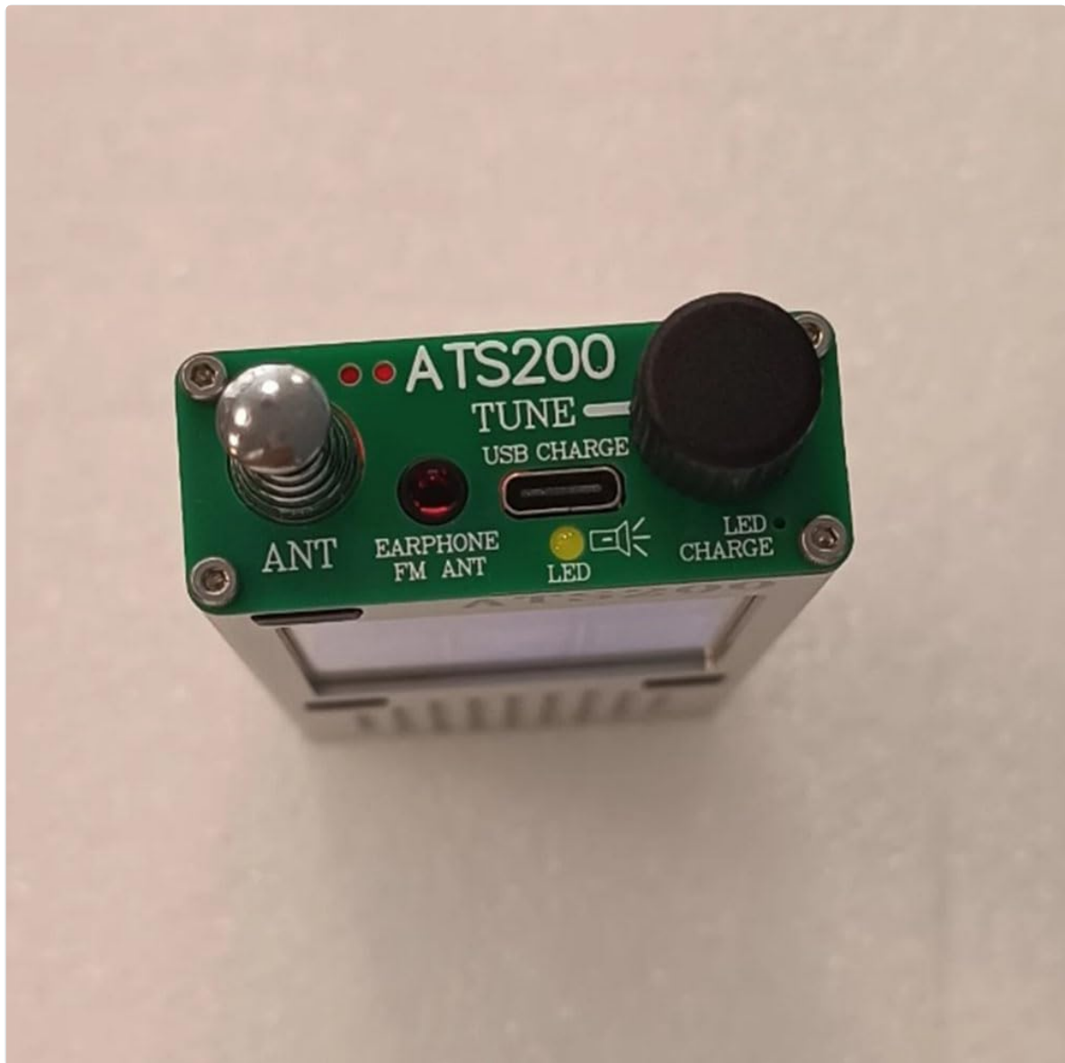
Figure 2: Top view of the ATS200, highlighting the USB-C charging port, tuning knob, and antenna connection.
