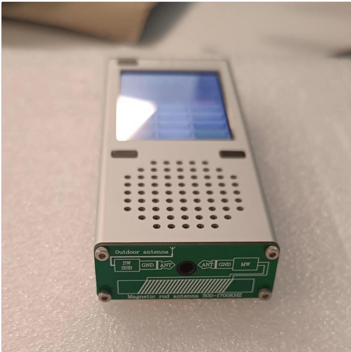
Figure 3: Bottom view of the ATS200, showing the external antenna interfaces for SW/SSB, MW, and a general antenna port.
