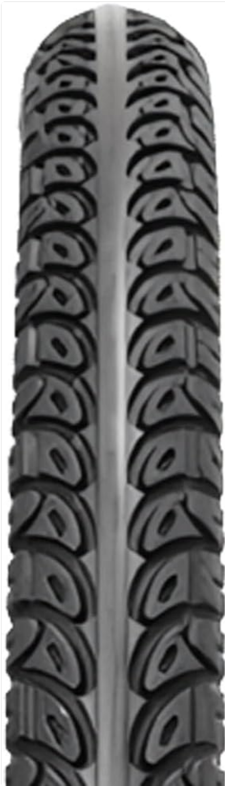
Figure 3.2: Detailed view of the Shinko SR024 tire tread. The image highlights the deep groove structure and the independent pattern of the side blocks, designed for improved grip.
