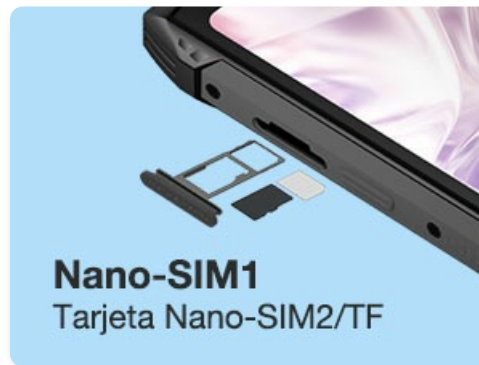
Figure 2.1: Illustration of the Nano-SIM and TF card tray, showing how to correctly insert the cards into the device.
