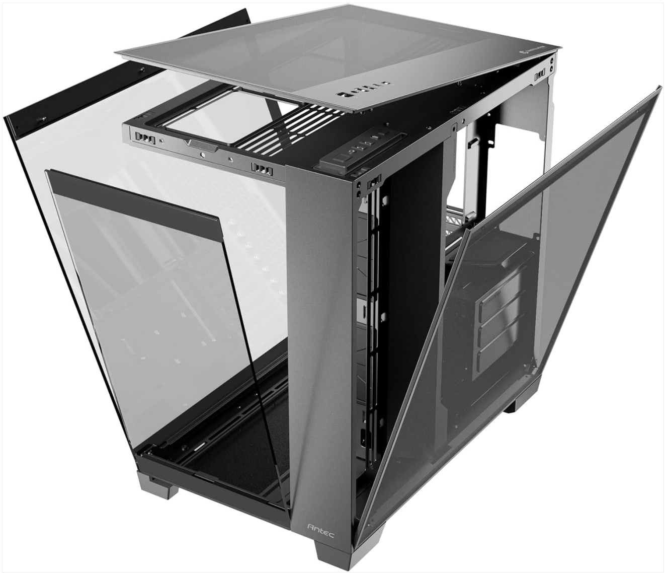
Figure 4: Side panel removal for easy access.
