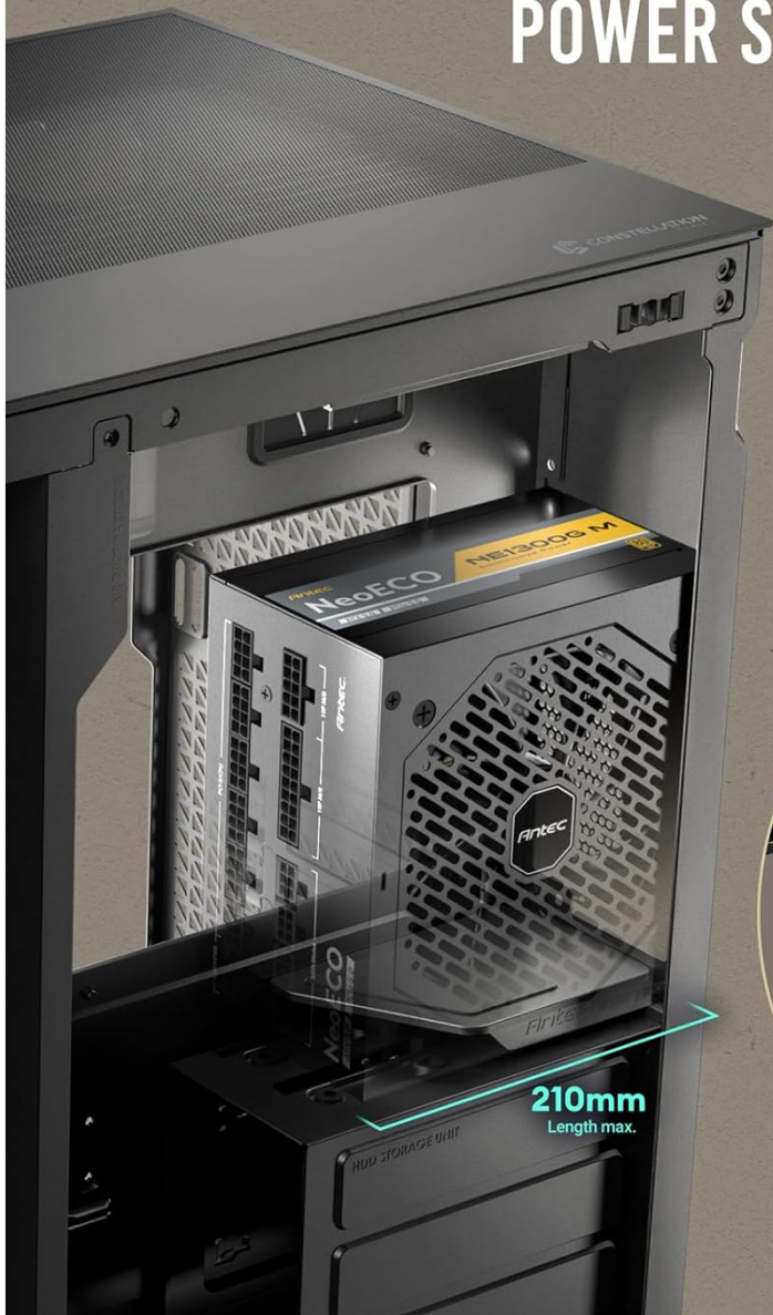
Figure 8: Power supply unit installation.
