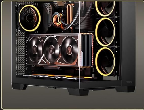
▲ Vertical Graphics Card Installation
