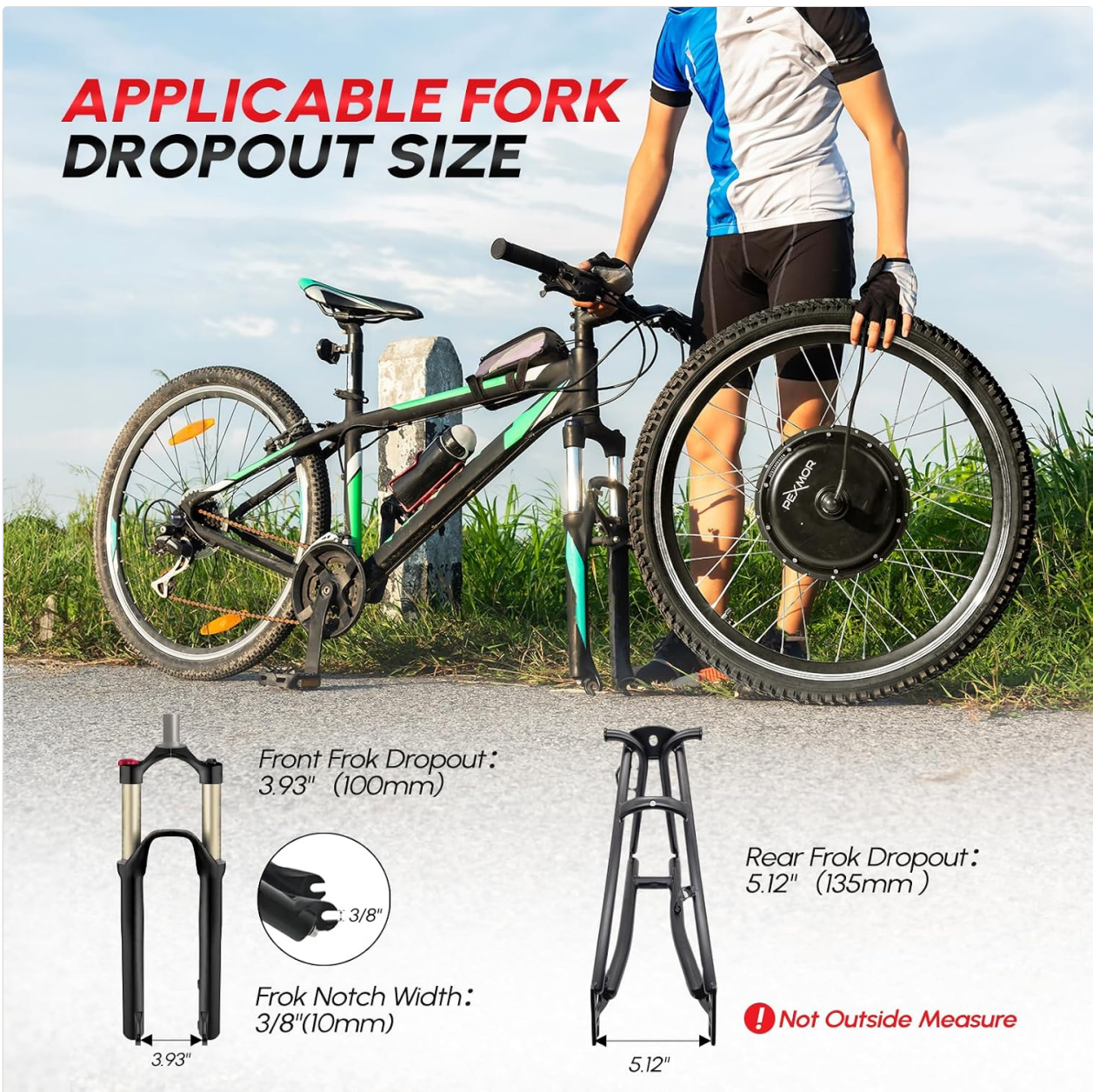
Image: Diagram showing applicable front and rear fork dropout sizes.
