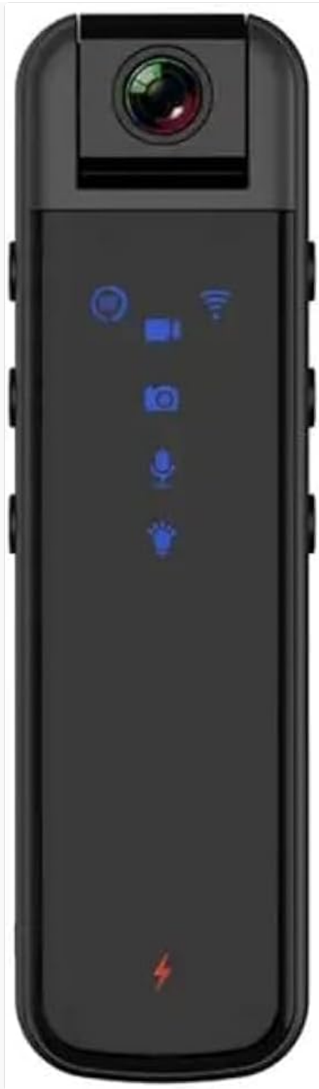
Figure 3.1: Front view of the Gulflink CS05 Camera. This image displays the camera's main body, the rotatable lens at the top, and the indicator lights on the front panel.
