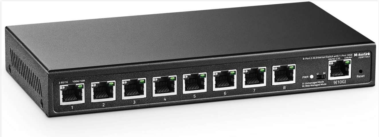
Figure 4.1: Front view of the MokerLink 8 Port 2.5G Ethernet Managed Switch, showing all 8 x 2.5G ports, 1 x 10G uplink port, PWR LED, and the U/M mode switch.
