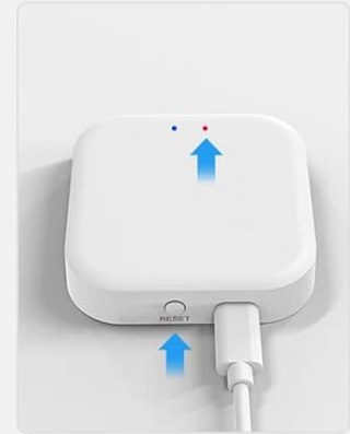
Step 4: Press and hold the "reset" button for 5 seconds until the red light flash fast, then pairing
