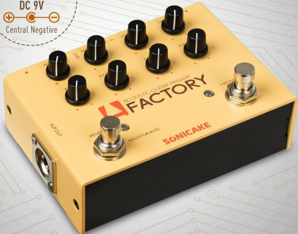
Image: The A-Factory pedal illustrating the 9V DC center-negative power input requirement.
