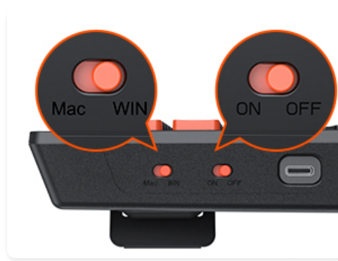
Image: Close-up of the keyboard's Mac/WIN compatibility switch and the main ON/OFF power switch.
