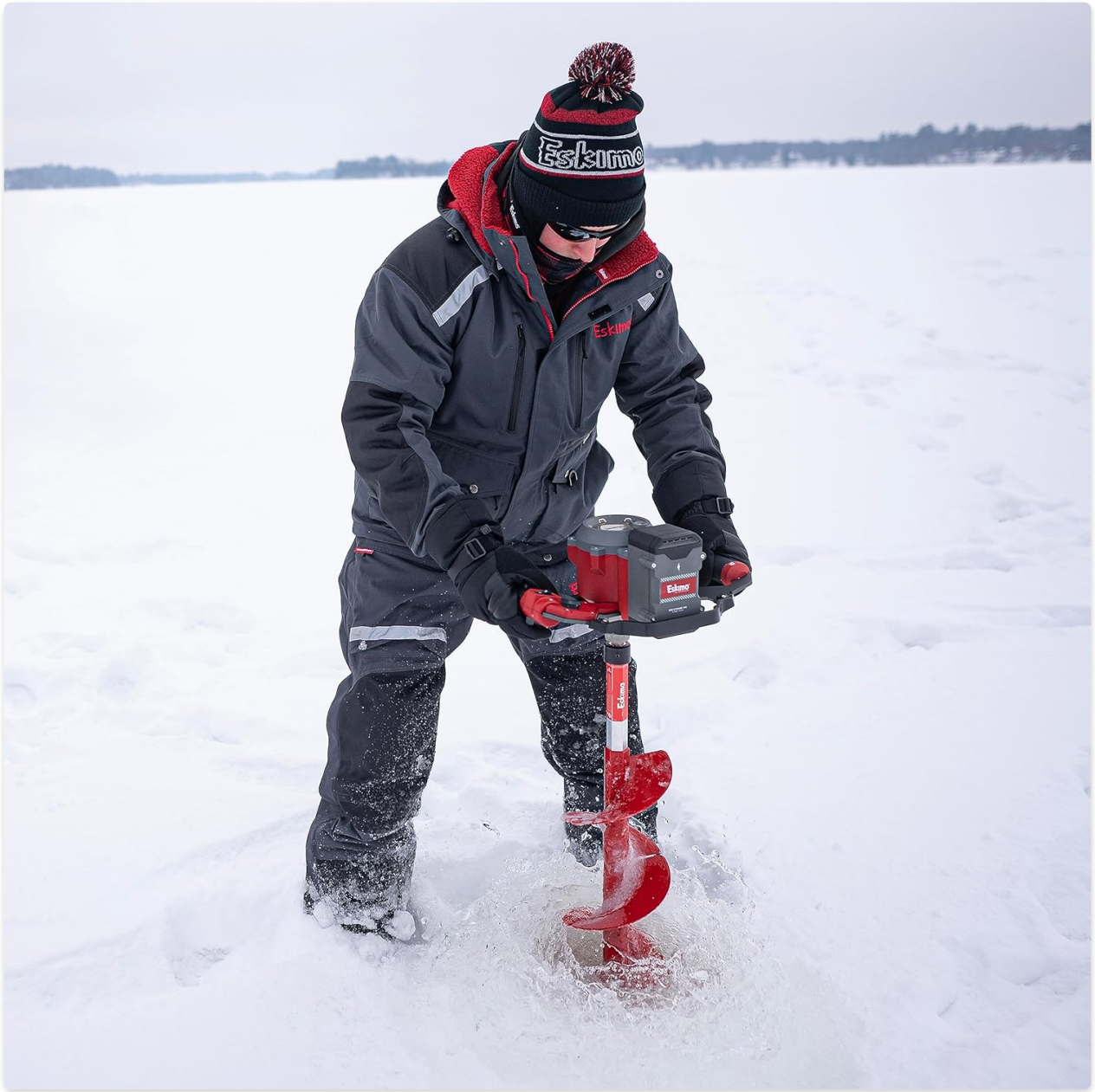
Figure 3: Operating the Eskimo E40 auger to drill an ice hole.
