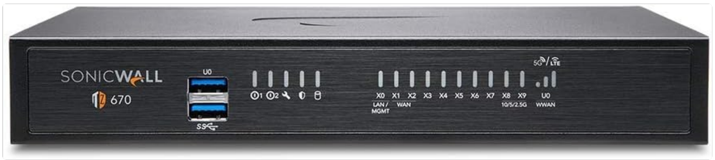
Figure 1: Front Panel of SonicWall TZ670
