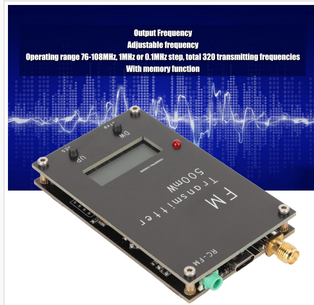
Figure 5.1: The transmitter displaying output frequency information. Note: The operating range is 88-108MHz as per specifications, though some images may indicate 76-108MHz.
