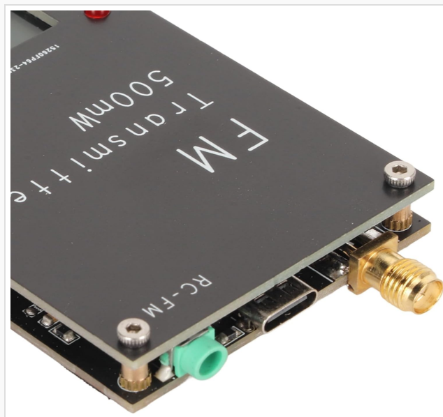
Figure 3.2: Close-up view of the 3.5mm audio input and USB-C power port.
