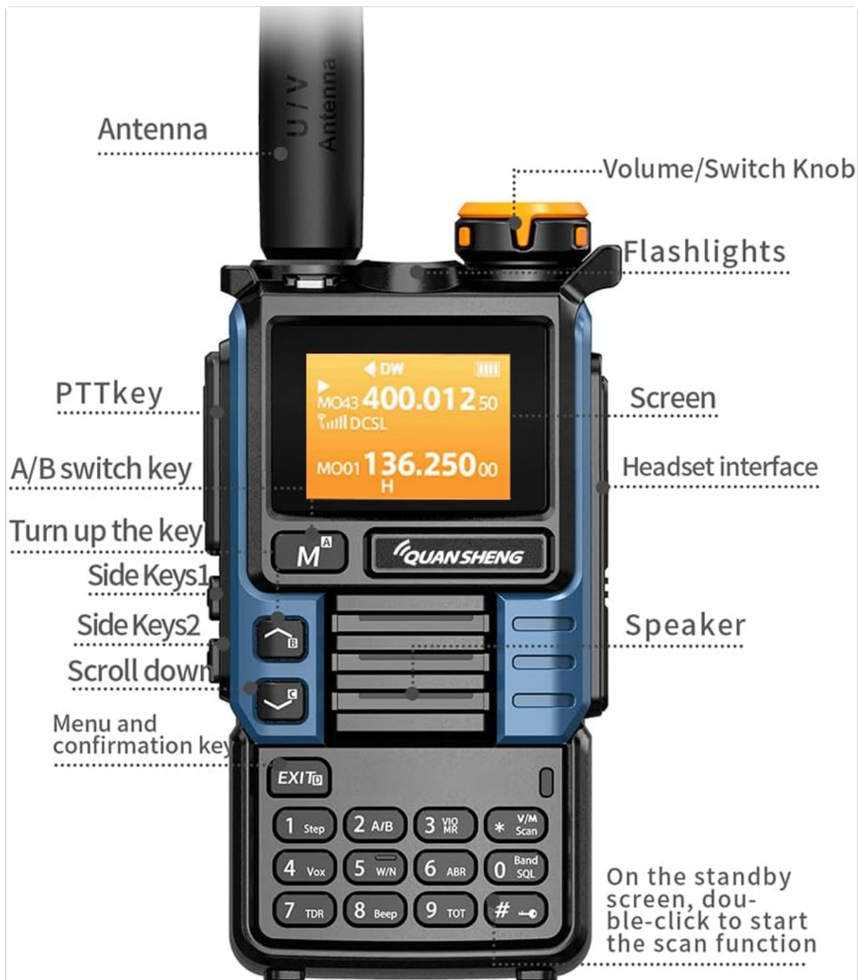
Figure 2: UV-K5(99) Component Diagram
