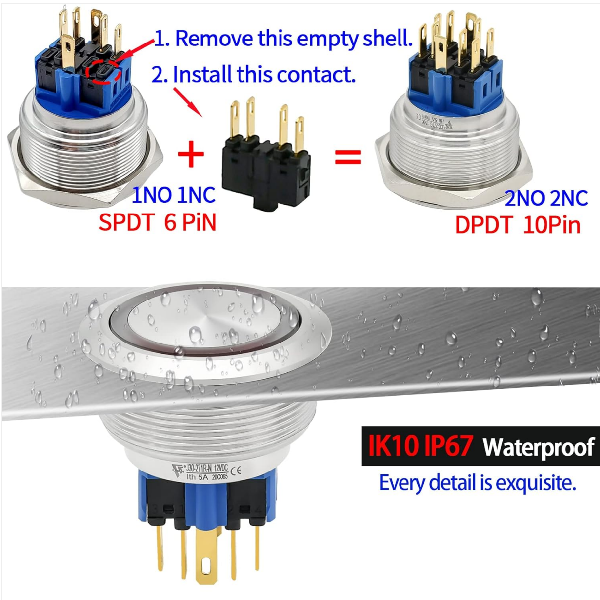
Figure 4: Instructions for converting the switch from its default 1NO1NC (SPDT) configuration to 2NO2NC (DPDT) by installing the provided spare contact. This increases the number of independent circuits the switch can control.
