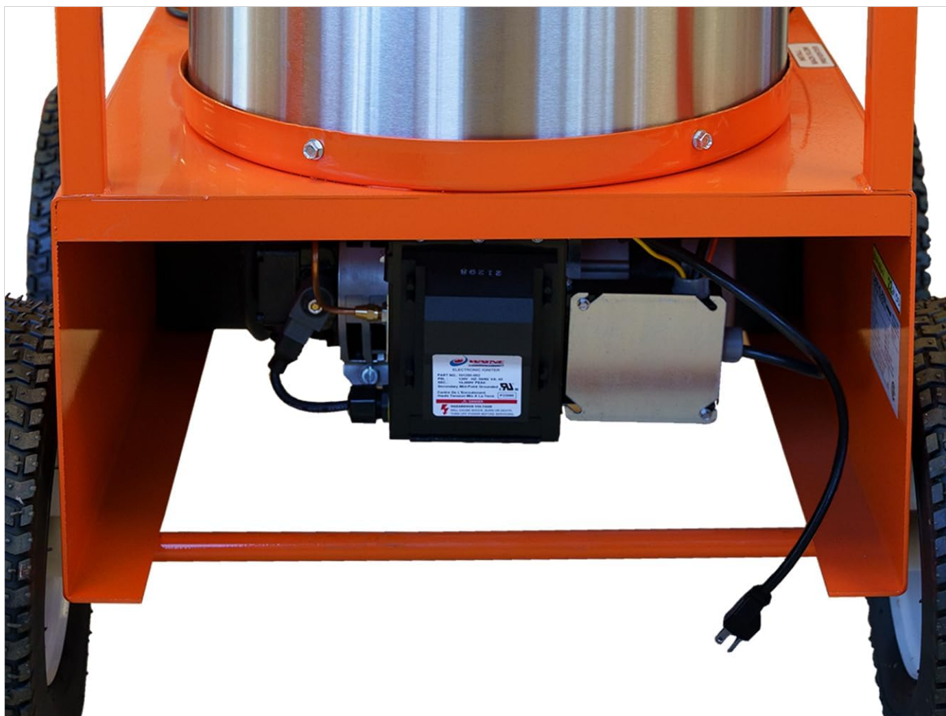
Image 5.2: Underside view of the pressure washer, showing the 120V oil-fired burner assembly and electrical connection.
