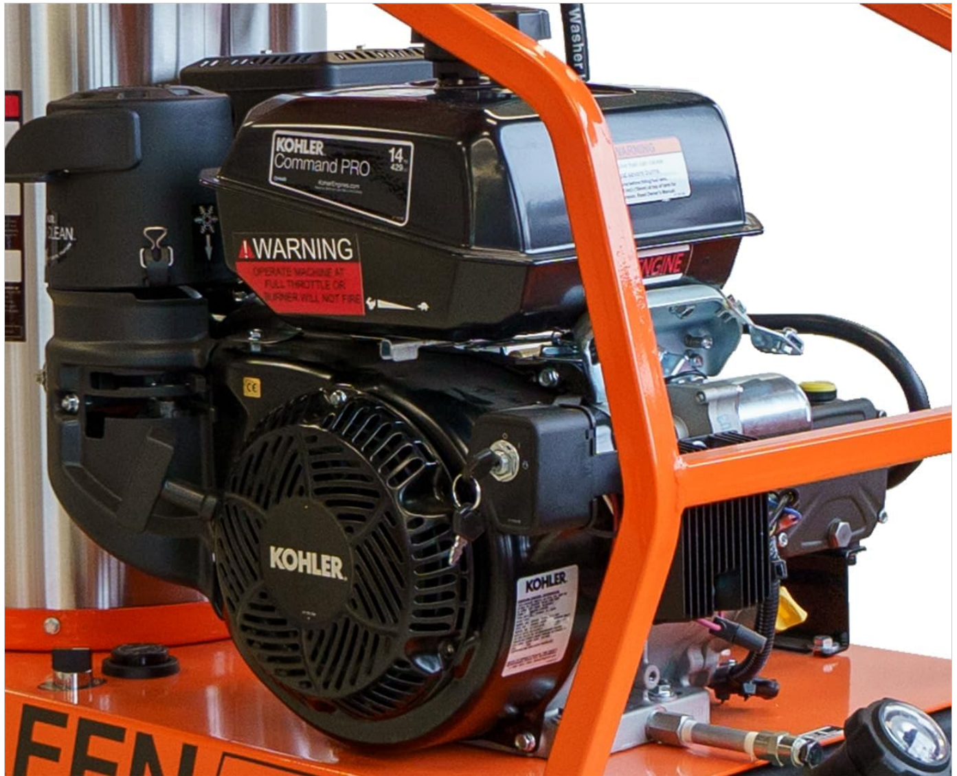
Image 5.1: Close-up view of the 14 HP Kohler engine, indicating areas for oil checks and air filter access.
