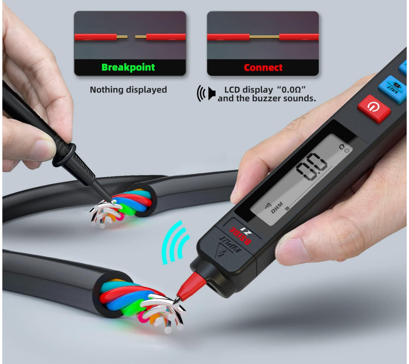
Figure 5.1: Performing a continuity test. The multimeter beeps and displays "0.0" for a continuous circuit.
