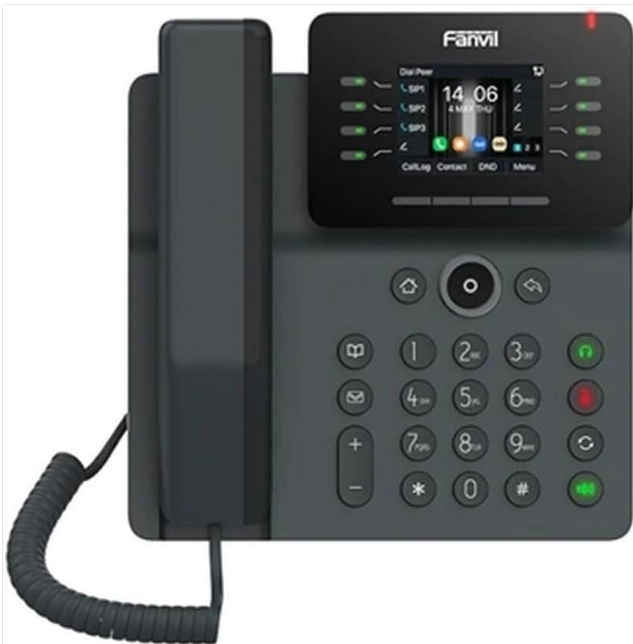
Figure 1: Front view of the Fanvil V63 VoIP Phone, showcasing its display, keypad, and handset.
