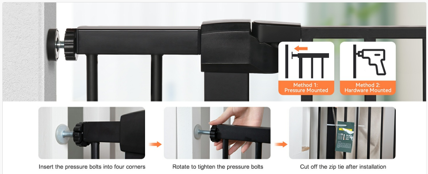
Image 3.2: Steps for pressure mounted installation.
