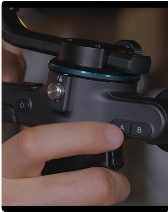
Figure 2: The quick-release system allows for rapid transition to vertical shooting.
