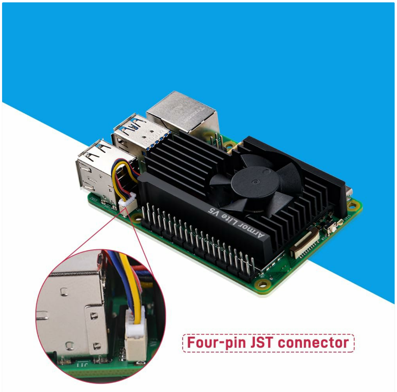
Figure 3.3: Detailed view of the 4-pin JST connector on the Raspberry Pi 5, where the cooler's fan cable is connected.
