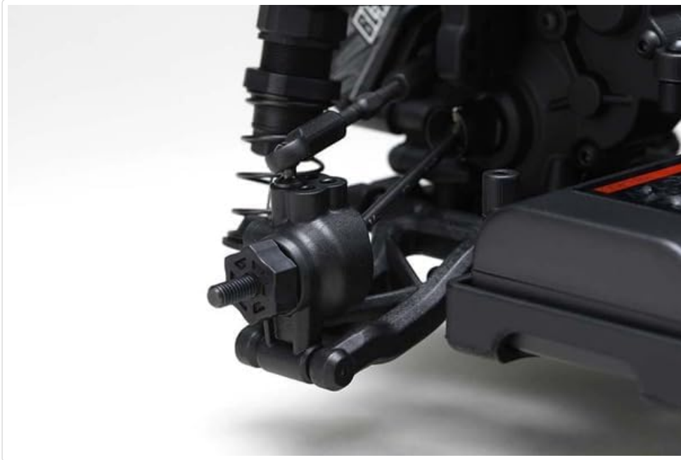
Figure 3.5: The rear hub and knuckle assembly, which connects the wheels to the chassis and houses the rear axles.
