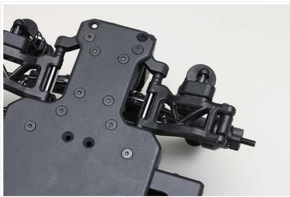
Figure 3.6: An underside view of the chassis, illustrating the layout of the suspension components and the central drive shaft area.
