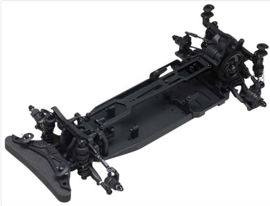
Figure 2.1: Fully assembled Yokomo Rookie Drift RD2.0 chassis, showcasing its layout and components.
