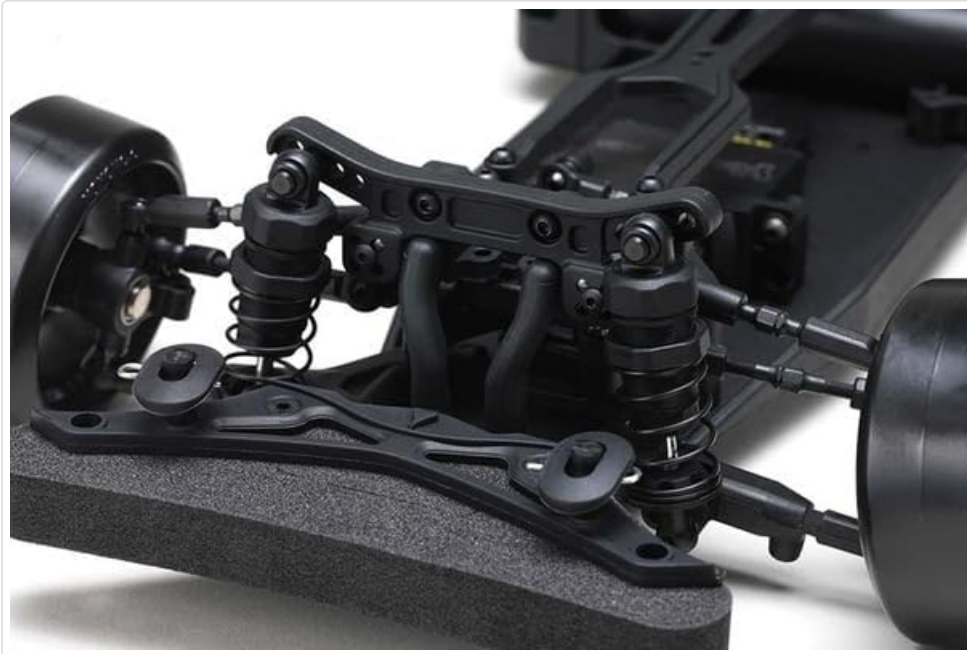
Figure 3.3: The front suspension system, showing the arms, shock towers, and their attachment points to the chassis.
