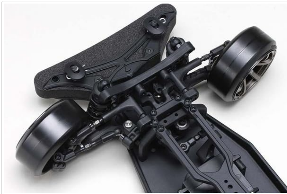
Figure 3.1: Detailed view of the front suspension and bumper assembly, highlighting the steering components and shock mounts.
