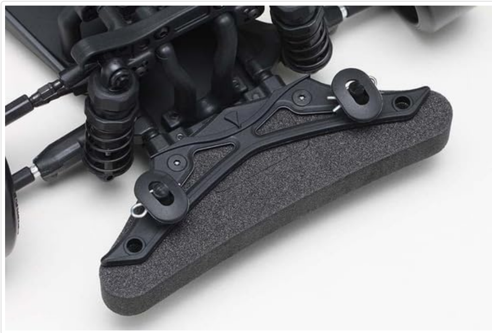
Figure 3.2: Close-up of the front bumper, designed for impact absorption and chassis protection.
