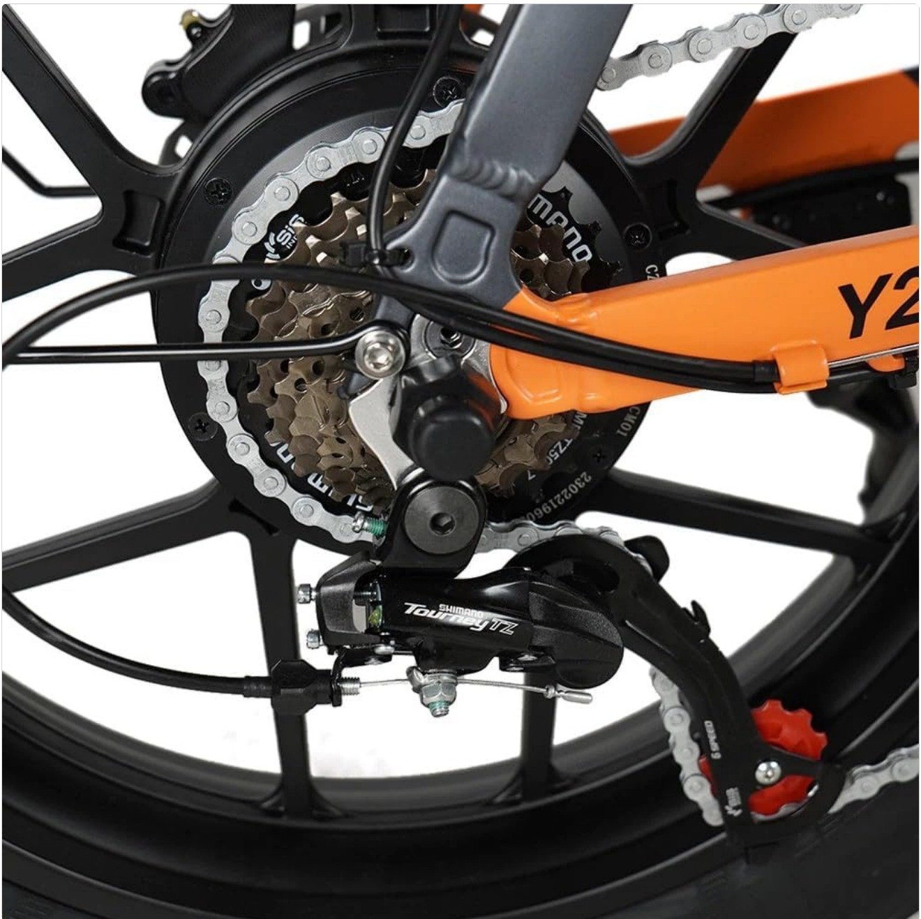
Image: Close-up of the VAKOLE Y20 PRO's rear wheel, showing the Shimano Tourney TZ derailleur and 7-speed cassette, responsible for gear changes.
