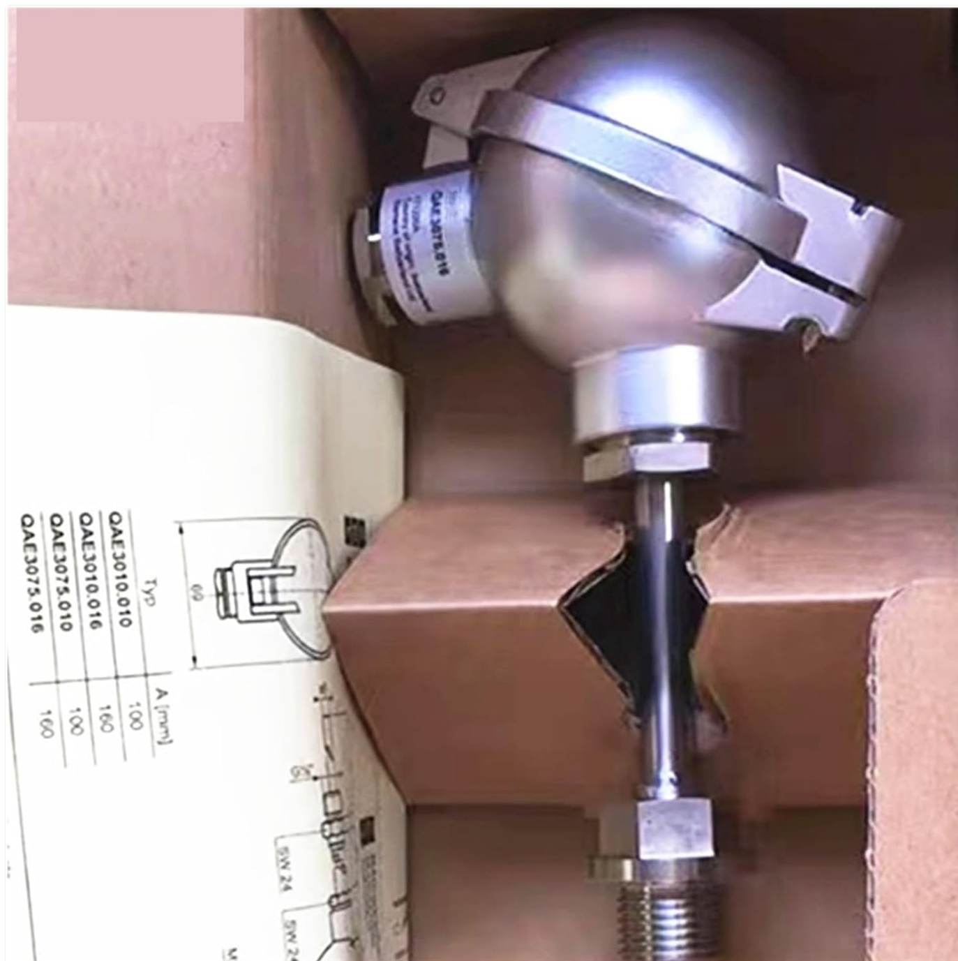
Figure 3: Close-up of the sensor's connection head. This view highlights the area where electrical connections are made, which is crucial for proper setup.
