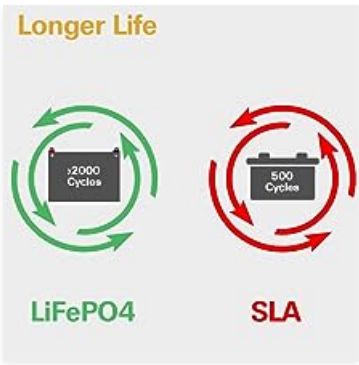
Image: Comparison graphic showing LiFePO4 batteries offering over 2000 cycles versus SLA batteries with approximately 500 cycles.
