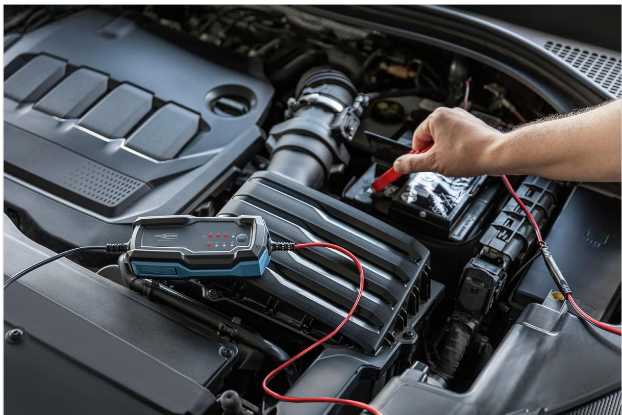
Figure 2: Example of connecting the charger to a car battery using battery clamps.
