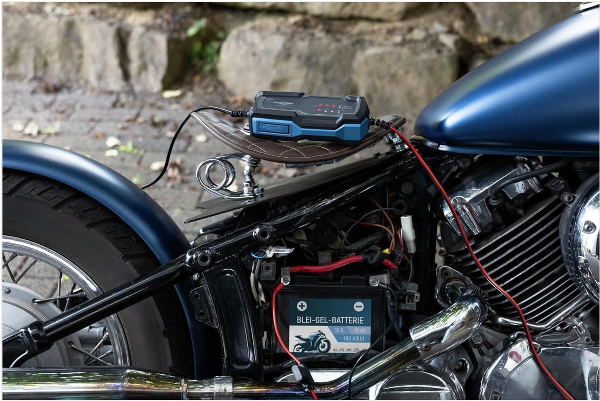
Figure 3: Example of connecting the charger to a motorcycle battery.
