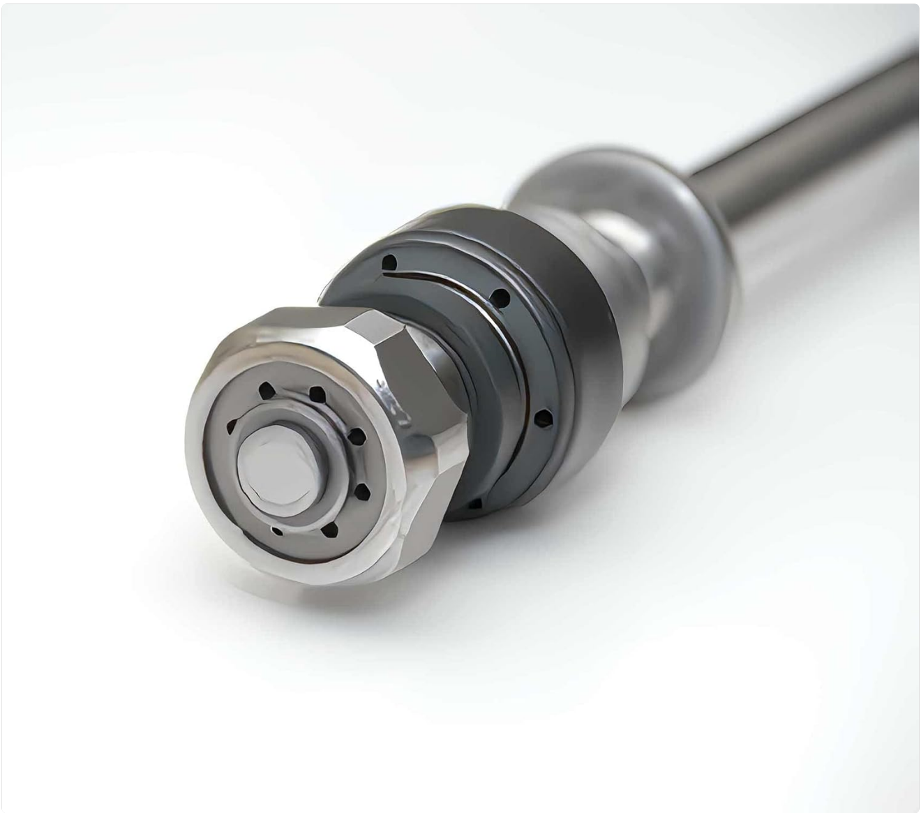
Image: Close-up of the threaded body and adjustment collar on the Cusco Touring A shock absorber. This mechanism allows for precise vehicle height adjustment.
