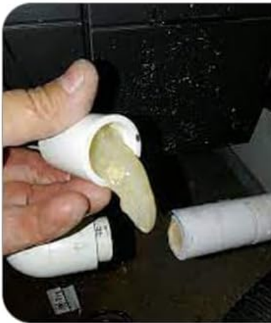
Figure 4.1: Illustration of Zooglea, a type of bacteria that thrives in dark, damp A/C drain lines, and factors contributing to its growth (Moisture, Nutrients, Environment).
