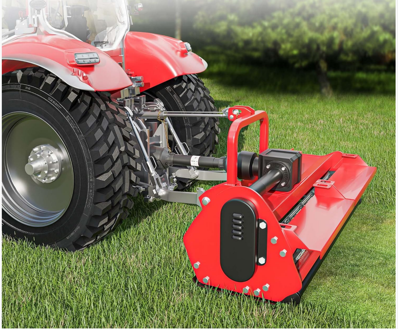
Figure 5: WilTec T5 PTO Shaft in operation with an agricultural implement.
