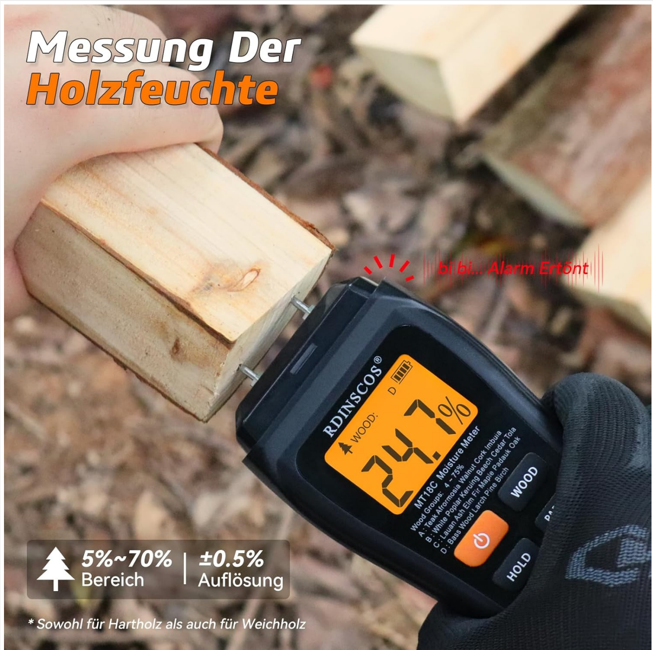
Figure 3: Taking a moisture measurement in wood.
