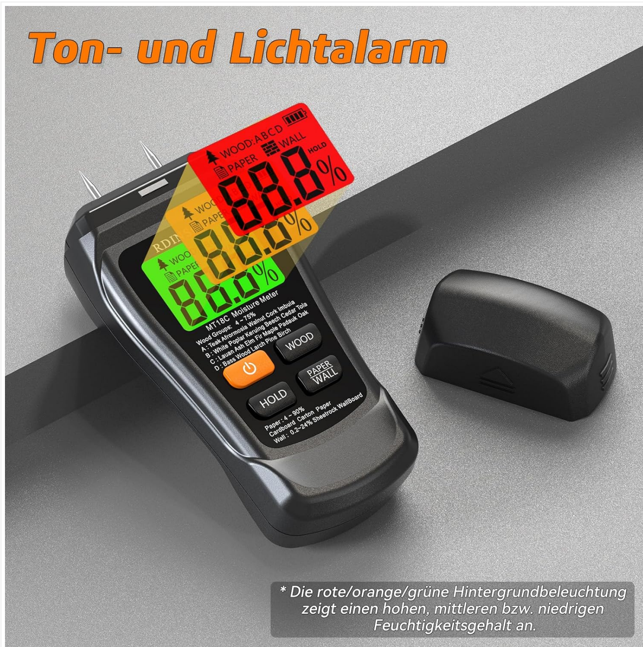
Figure 5: Visual and audible alarm indicators on the MT18C1 display.
