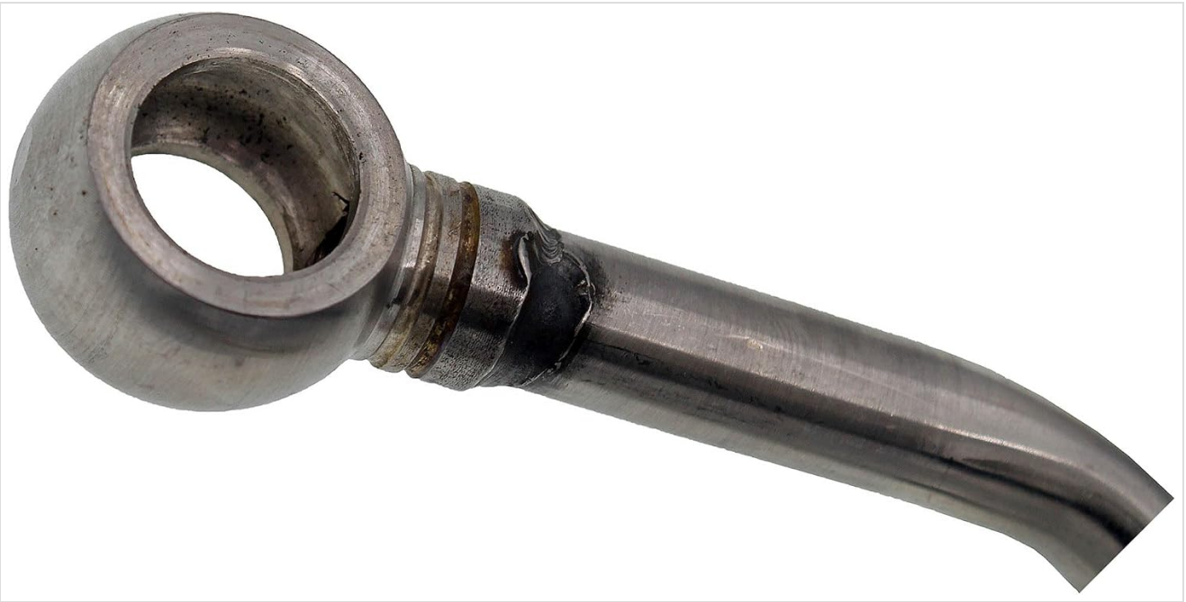
Figure 3: Detail of the other end of the coolant feed line, featuring a banjo bolt style fitting. Ensure new crush washers are used if required and the bolt is torqued to specifications.
