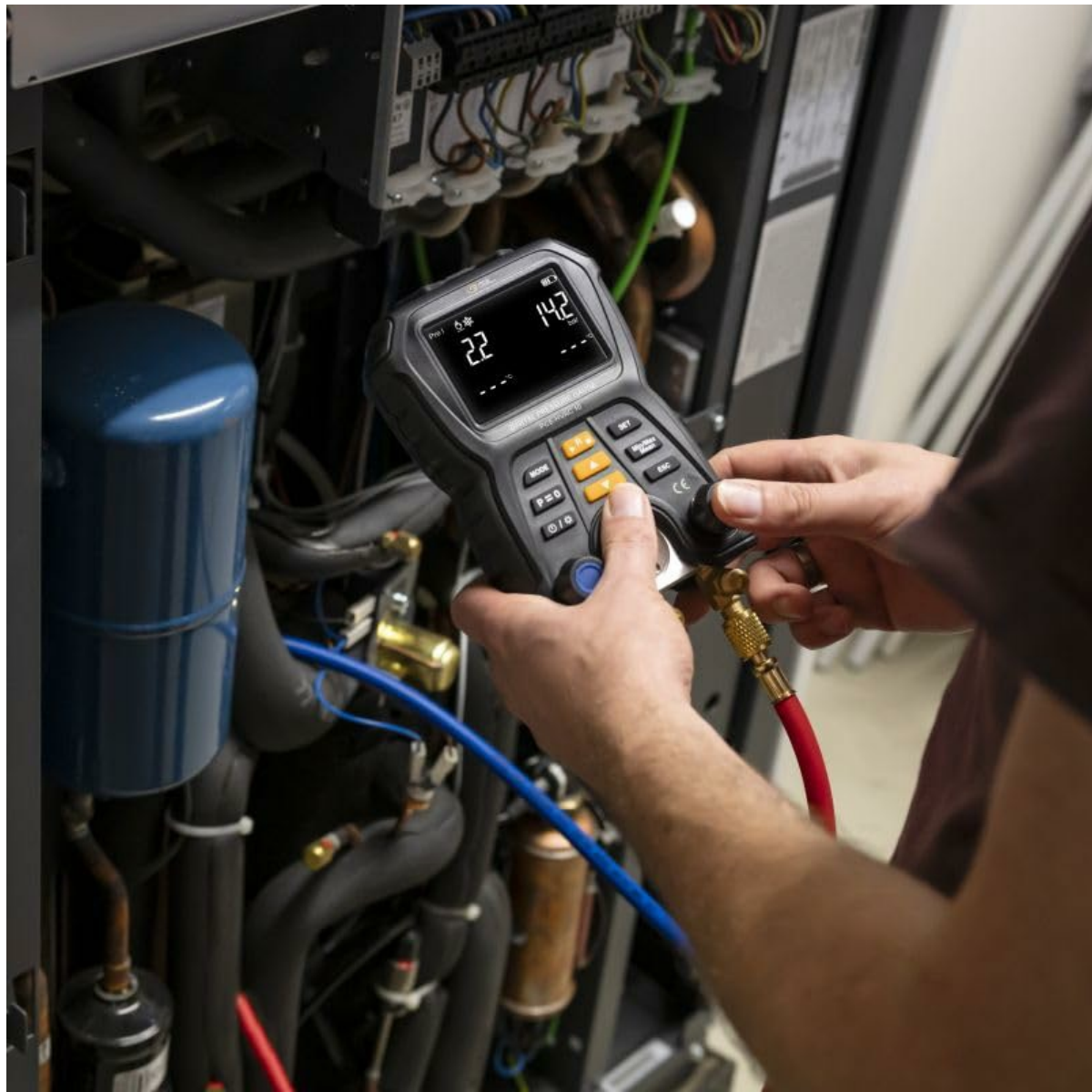
A technician using the PCE-HVAC 10 Digital Pressure Gauge to monitor an HVAC system, with hoses connected.
