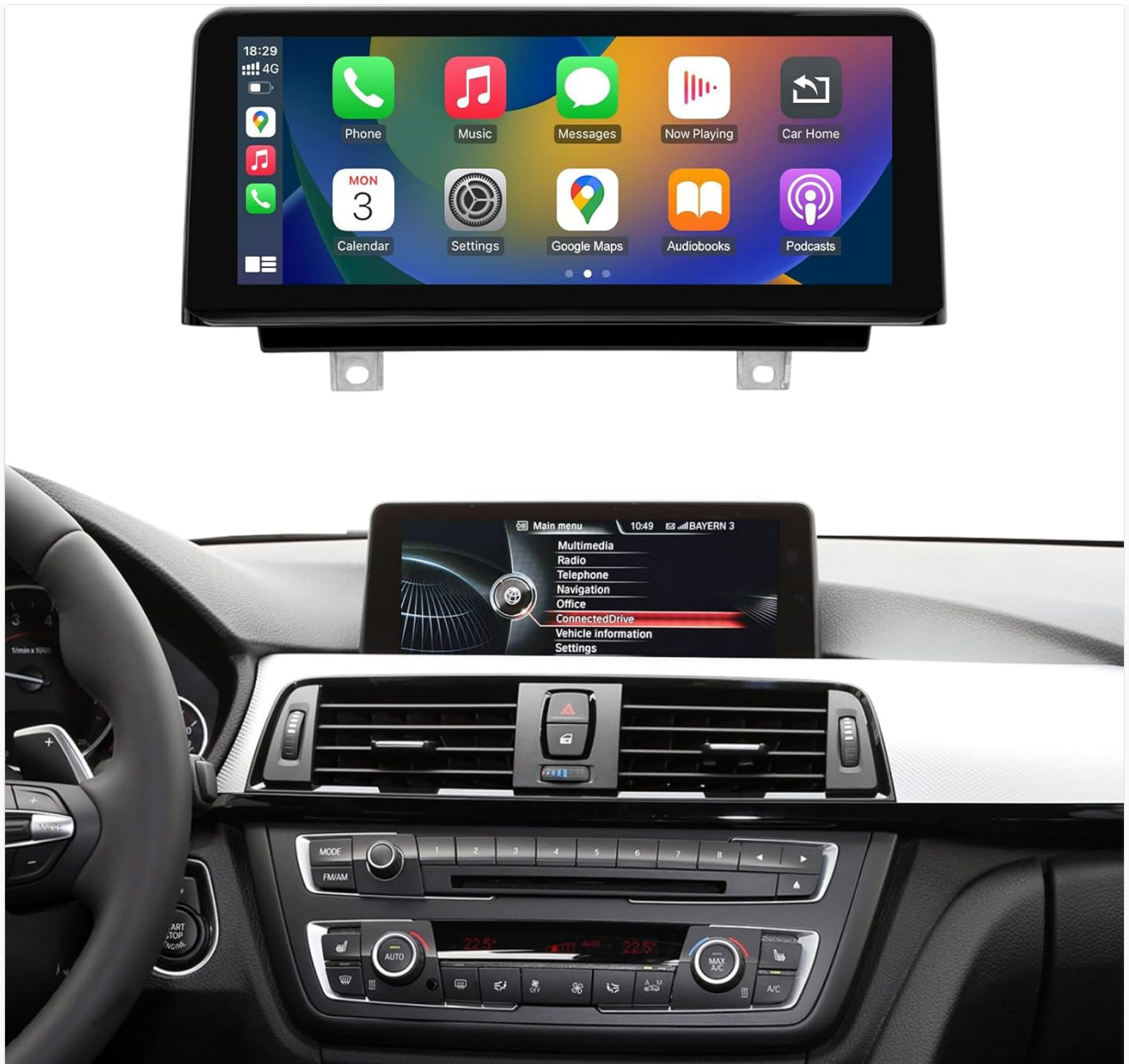
Figure 1.1: NINETOM 10.25 inch Touchscreen Multimedia Receiver installed in a BMW dashboard, displaying a CarPlay interface.
