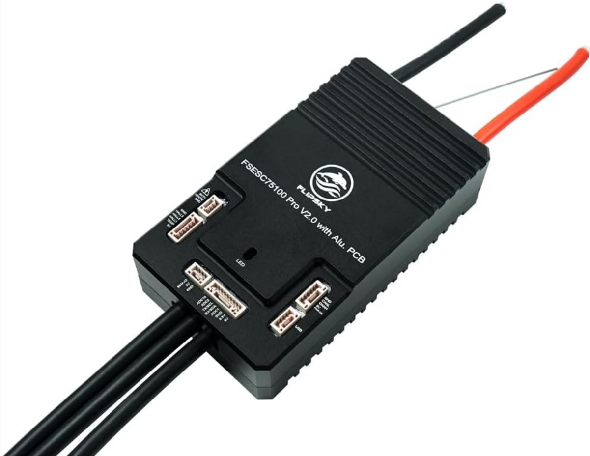
Figure 7: Visual representation emphasizing the 100A continuous current rating. It is critical not to exceed the specified voltage range to prevent damage to the ESC.
