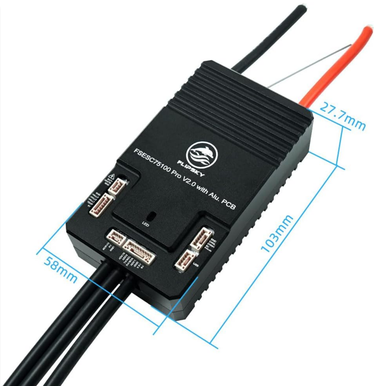
Figure 2: Physical dimensions of the ESC unit. The controller measures L103mm x W58mm x H27.7mm, indicating its compact design for various installations.
