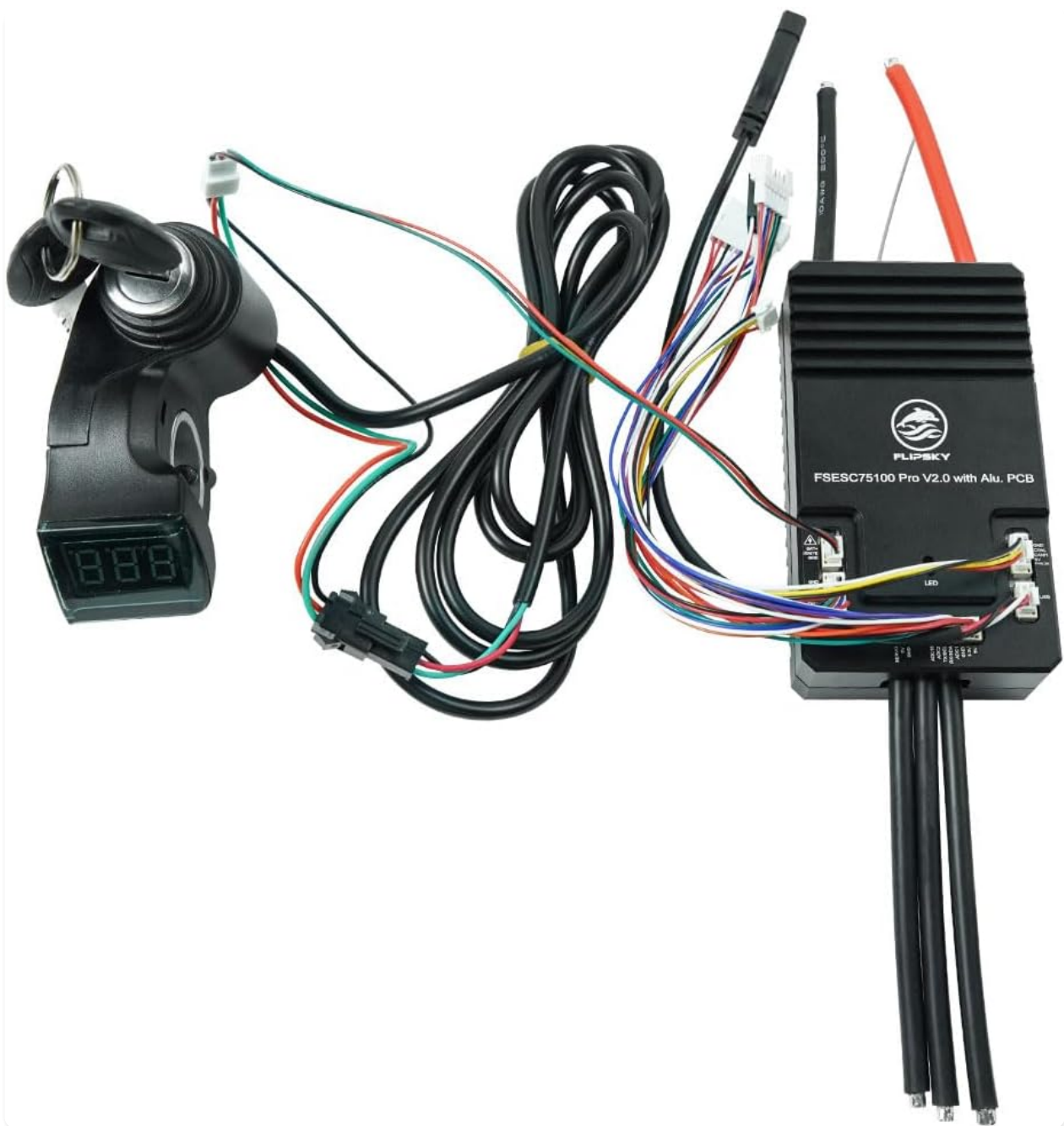
Figure 1: The FLIPSKY 75100 Pro V2.0 ESC controller, shown with its integrated key switch and various wiring harnesses for connection to battery, motor, and control signals.
