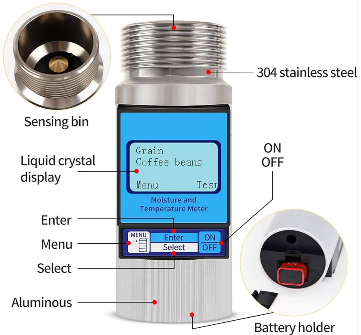
Figure 1: Overview of the JINGEDD Smart Grain Moisture Tester, highlighting its key components such as the sensing bin, liquid crystal display, menu, enter/select, and on/off buttons, and the battery holder.
