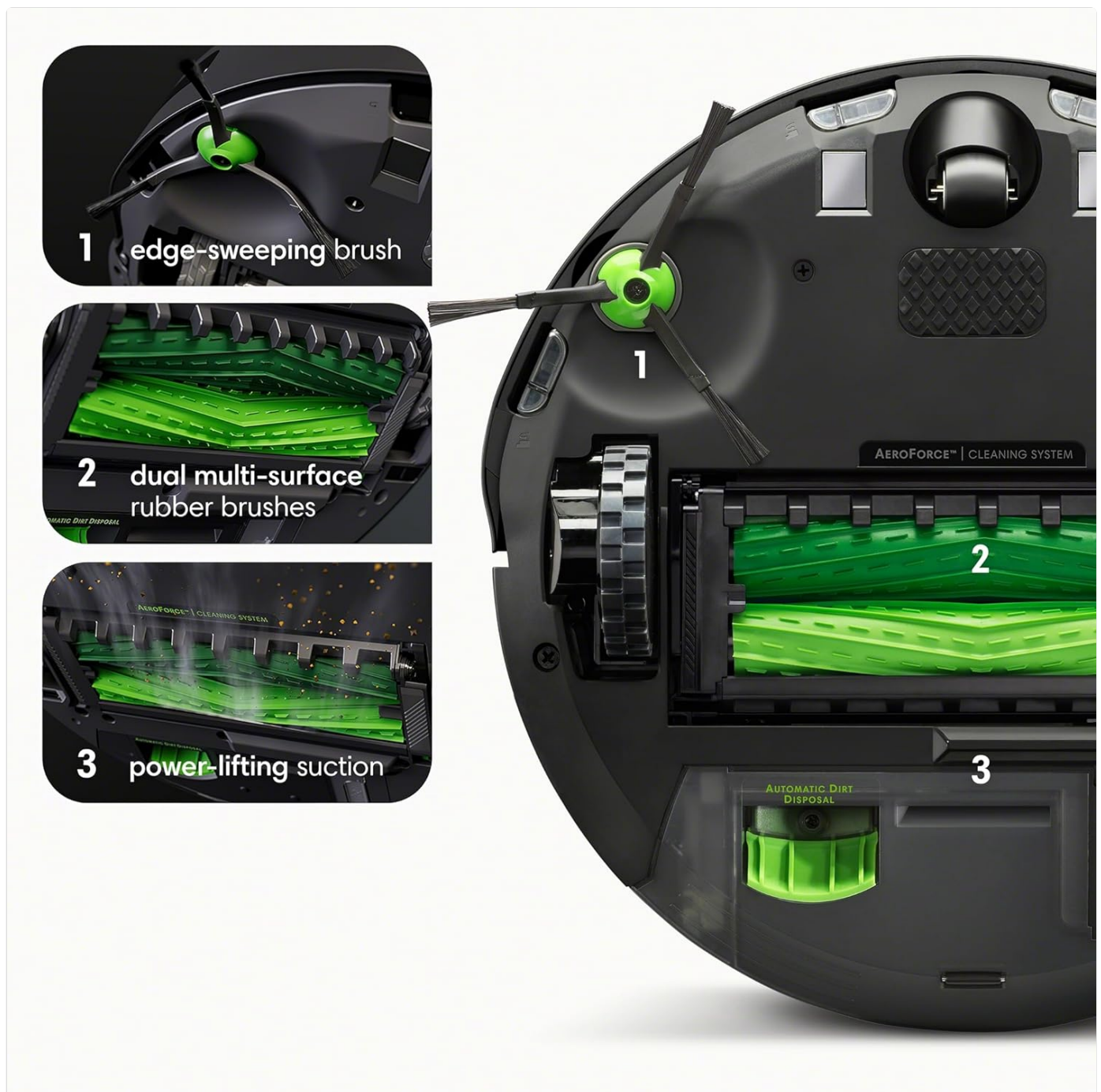
Image: A detailed view of the Roomba i3+ EVO's underside, highlighting its 3-stage cleaning system: edge-sweeping brush, dual multi-surface rubber brushes, and power-lifting suction.
