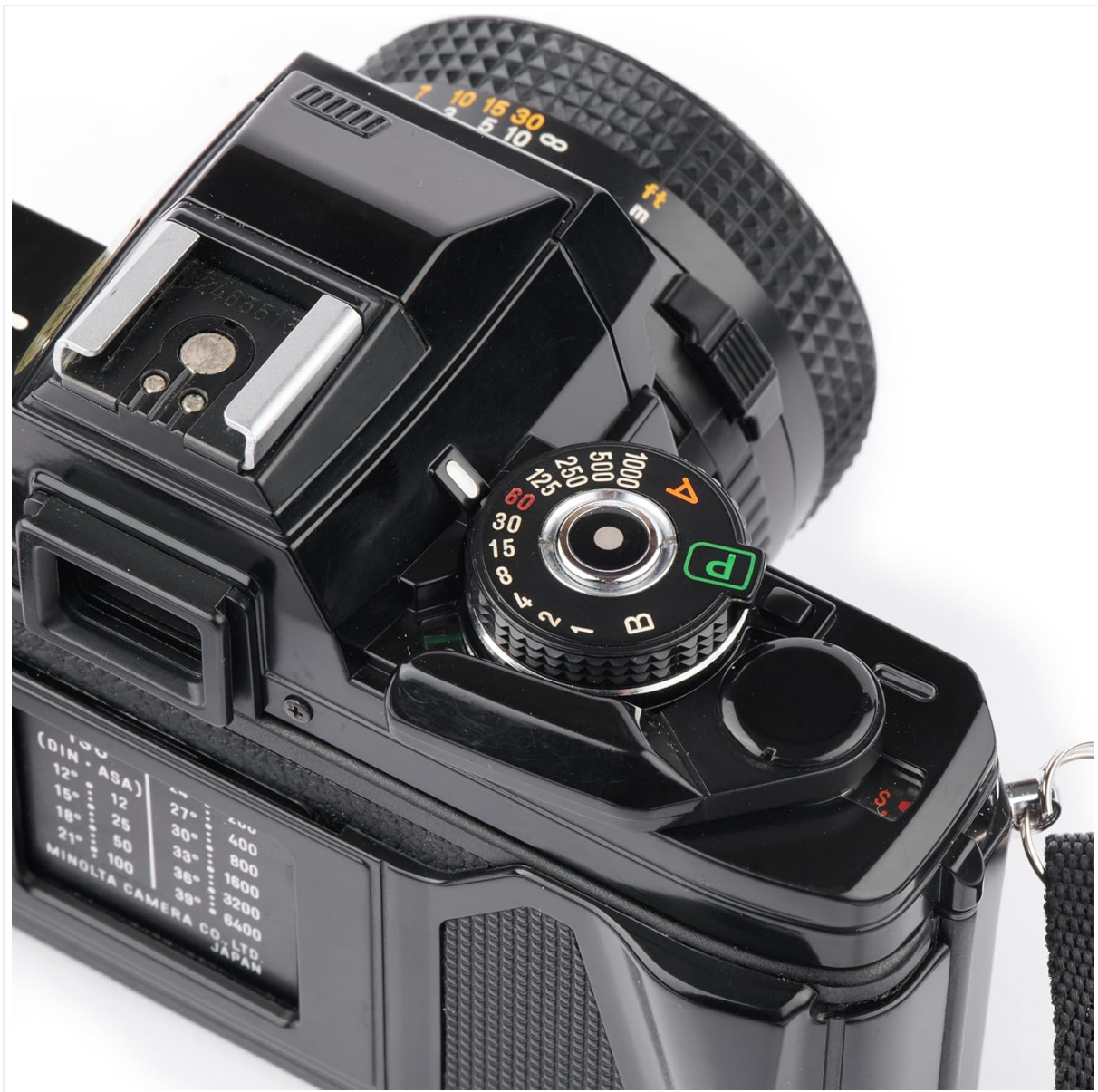
Figure 3.2: Top view of the Minolta X-700, showing the shutter speed and exposure mode dials.
