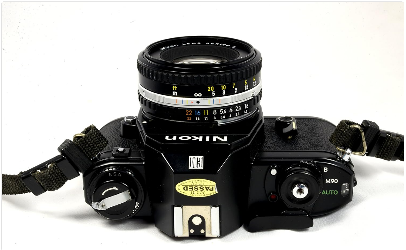
Figure 5: Top view of the Nikon EM, indicating the ISO/ASA dial.
