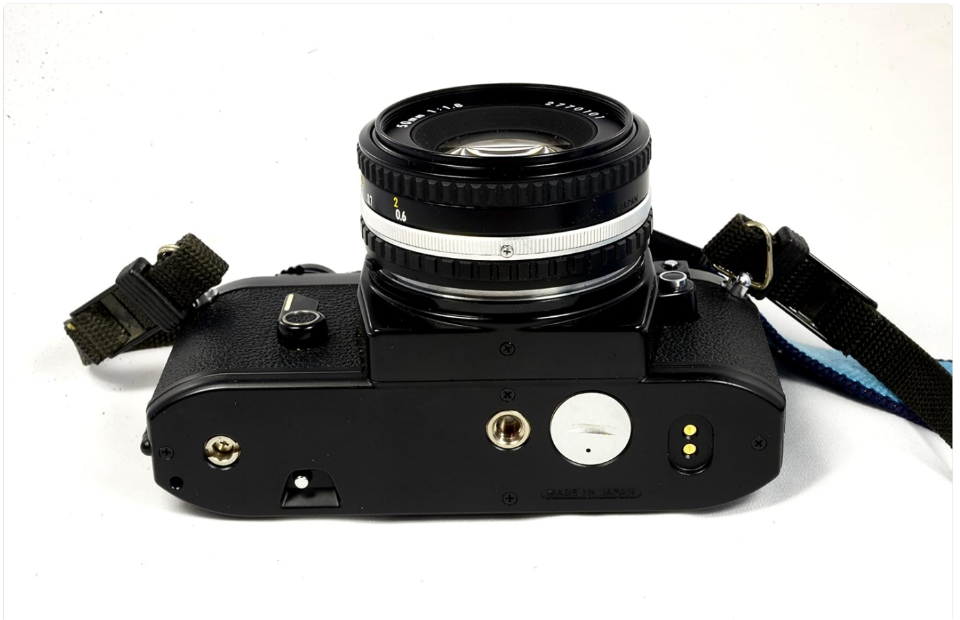
Figure 2: Bottom view of the Nikon EM, highlighting the battery compartment.
