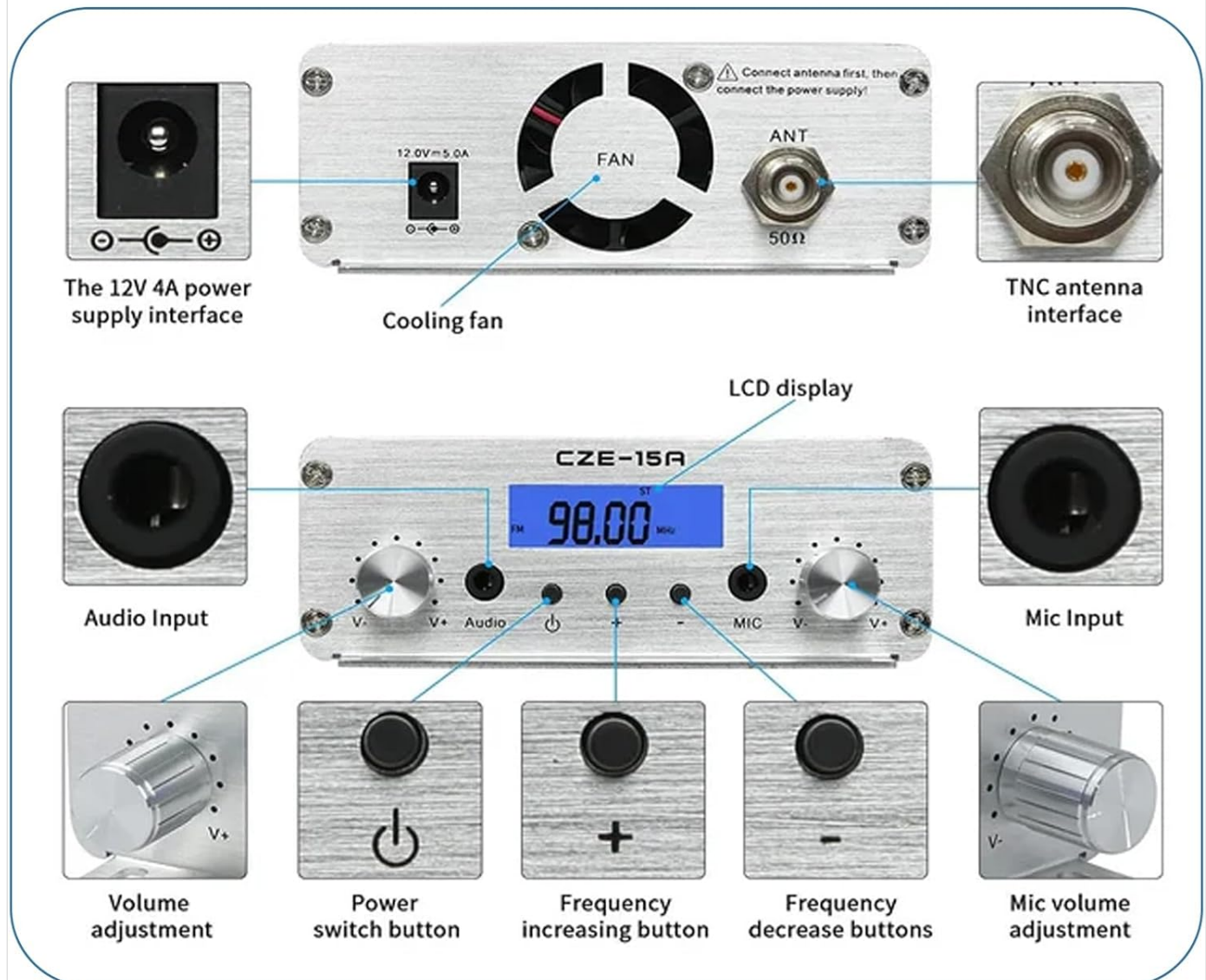
Figure 3: Detailed view of the CZE-15A transmitter's front and rear panel connections and controls.
