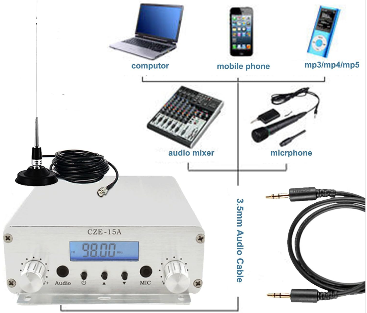
Figure 4: The 3.5mm audio input allows connection to various devices like computers, mobile phones, MP3 players, audio mixers, and microphones.
