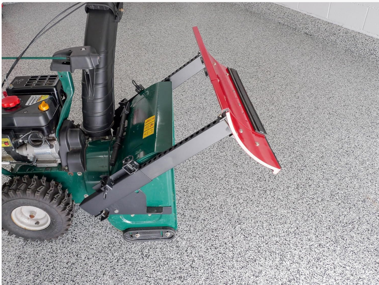
Image: The Throwerblade can be conveniently disconnected and folded for easy storage.
