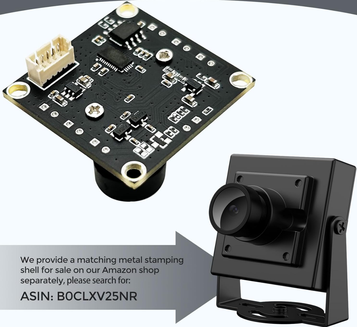
Figure 5: The camera module connected as a plug-and-play USB device.
