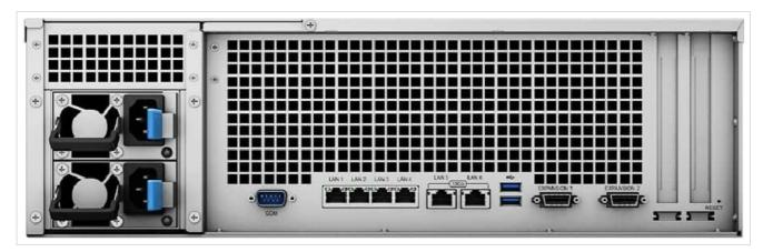
The rear panel includes dual redundant power supply units, four RJ-45 1GbE LAN ports, two RJ-45 10GbE LAN ports, two USB 3.2 ports, and two expansion ports for connecting Synology expansion units. A console port (COM) and a reset button are also present.
