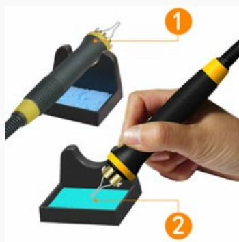
Image 4.3: Demonstrates moistening the sponge in the pen stand for cleaning the pen tip.
