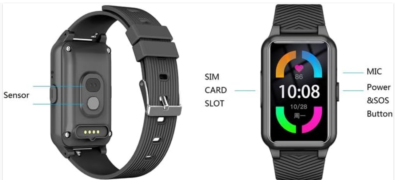
Figure 3.1: Smartwatch Components (Back and Front View)
