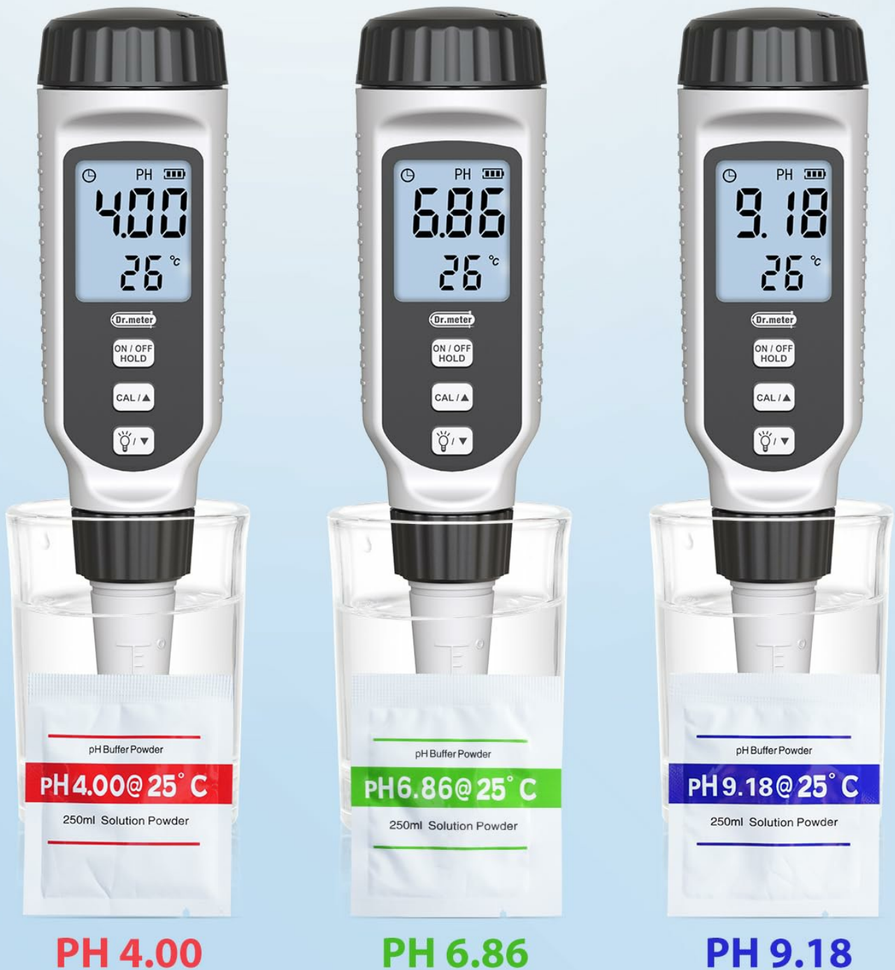
Image 6.1: Illustration of the 3-point calibration process using pH 4.00, pH 6.86, and pH 9.18 buffer solutions.
