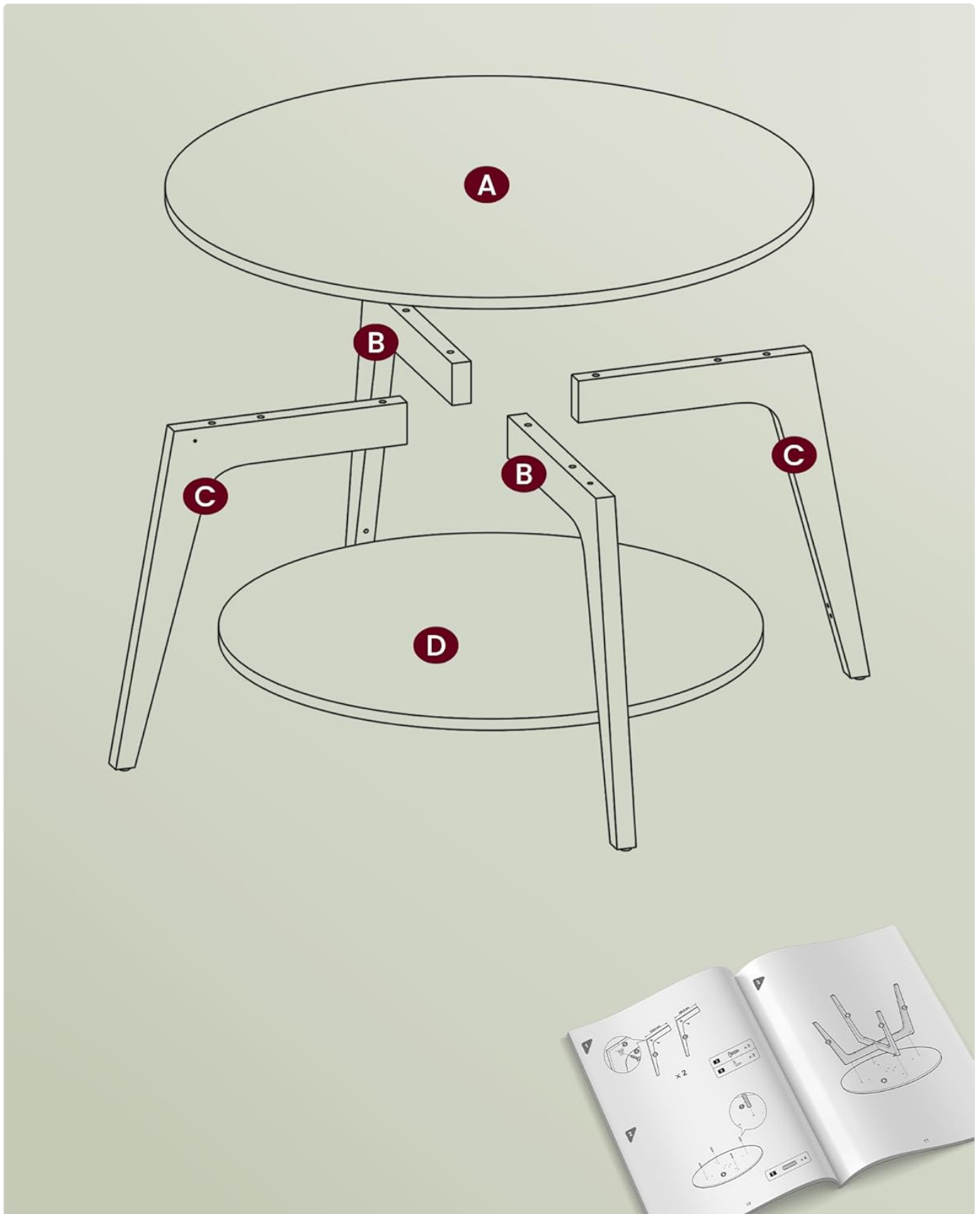
Image 2: Exploded view of the coffee table components, showing the tabletop (A), support brackets (B), legs (C), and lower shelf (D).
