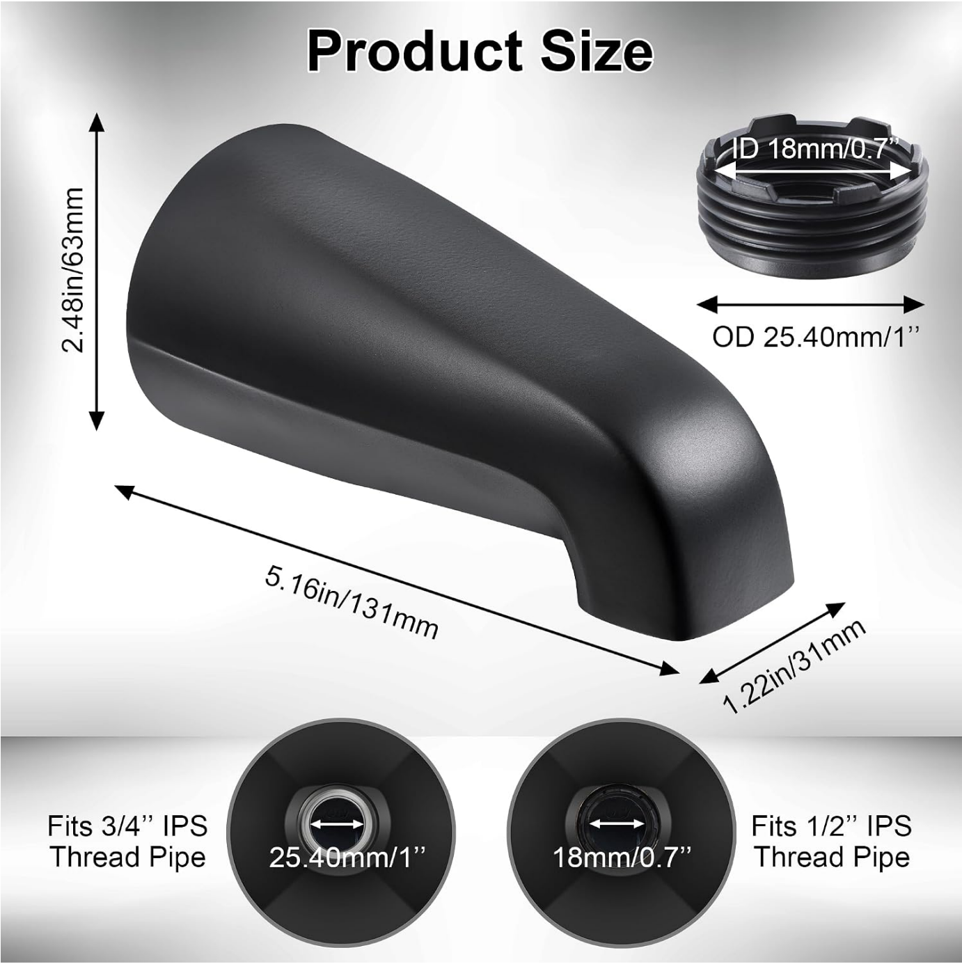
Image: This diagram provides detailed measurements of the tub spout, including its overall length, width, and the internal diameters for 1/2" and 3/4" IPS threaded pipes.
