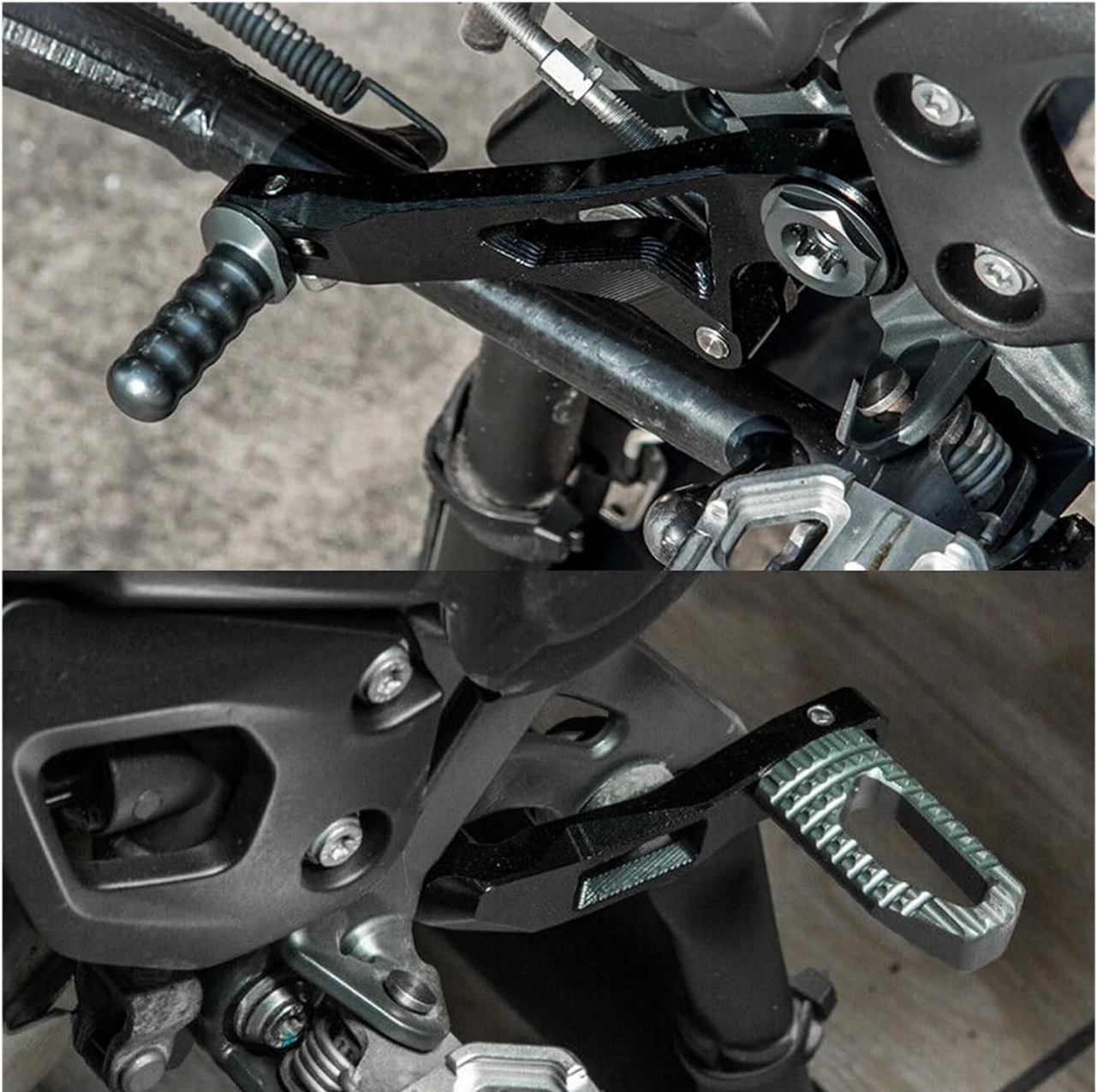
Figure 2.2: Close-up view of the SarUel Motorcycle Shift Lever and Footpeg installed on a BMW R1250GS. This image highlights the integration of the shift lever and footpeg with the motorcycle's existing components, demonstrating its fitment and appearance once installed.
