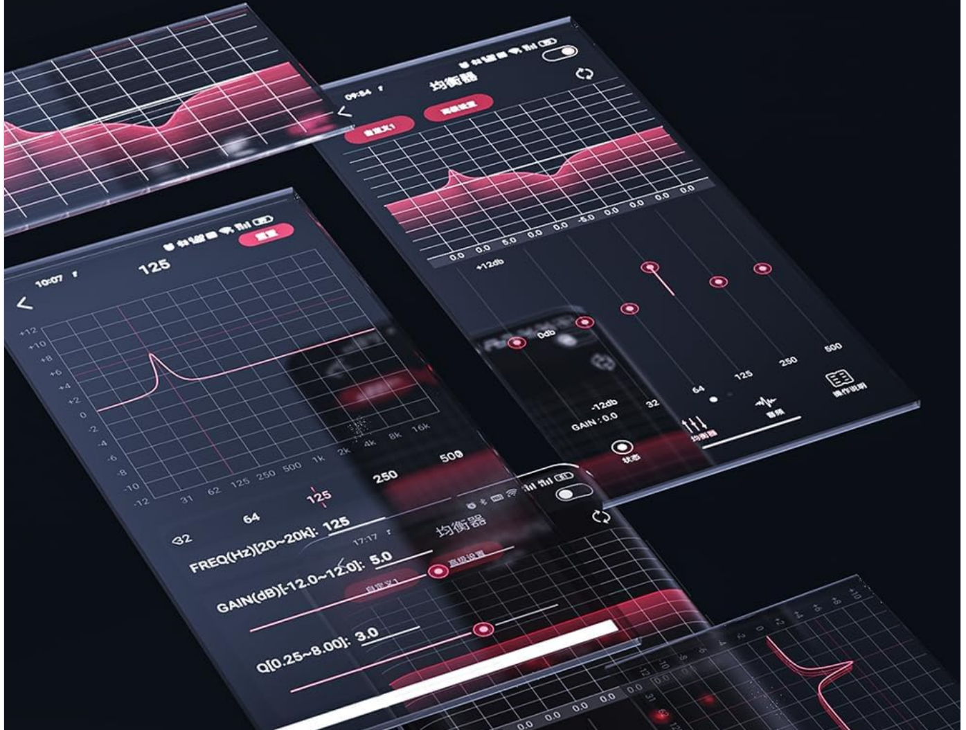
Image 4.5.1: Global PEQ Interface. This image displays the FiiO Q15's screen interface for the Global Parametric Equalizer, showing frequency, gain, and Q-factor adjustments.
