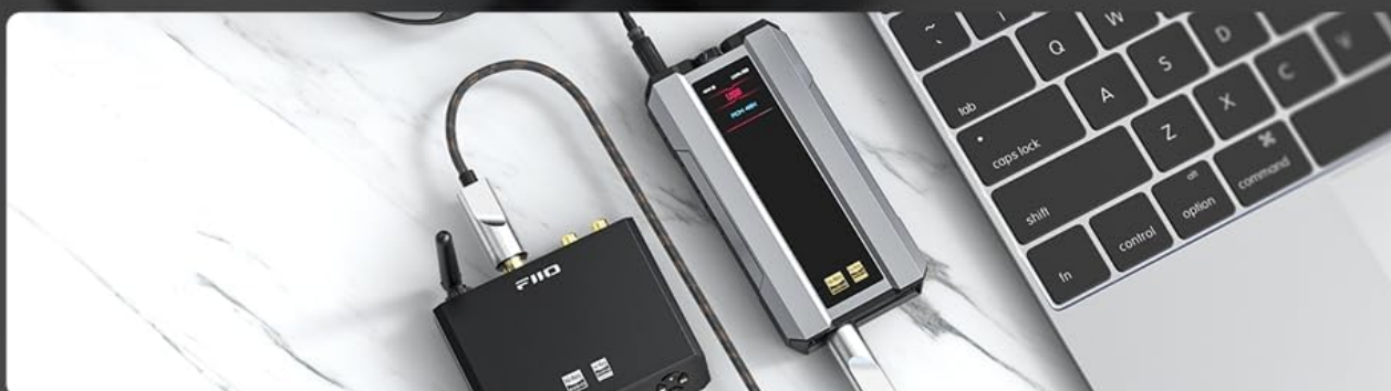
Image 3.2.1: Connectivity Examples. This image illustrates the FiiO Q15 connected to a laptop via USB, paired wirelessly via Bluetooth to
