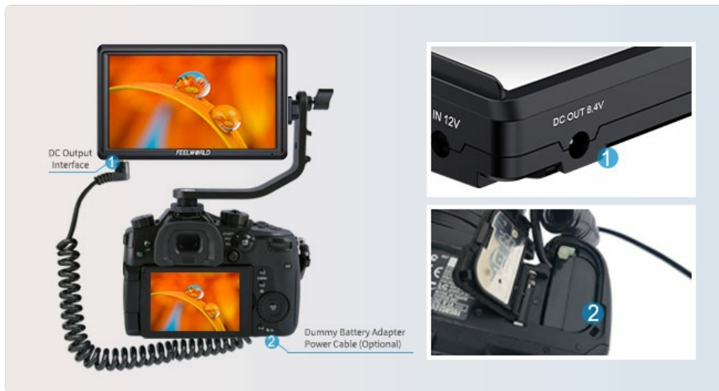
Figure 3.7: The FEELWORLD S55 V3 monitor connected to a camera, demonstrating its 8.4V DC output interface which can power the camera using a dummy battery adapter.
